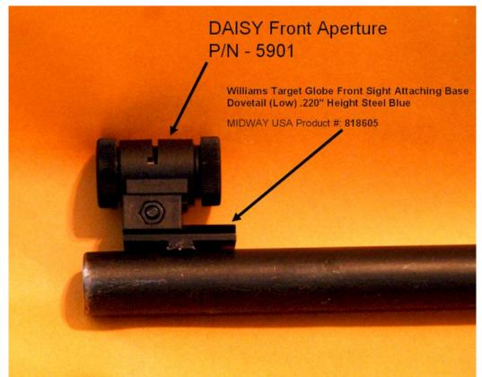
a) Removed the existing post sight and replaced with parts as shown below:
